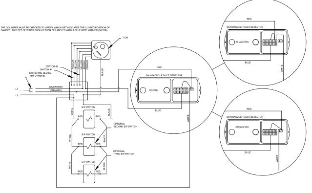
1. CONDUIT RUNS WHICH EXCEED 72" MUST HAVE GREEN GROUND WIRE. 2. FLEX CONDUIT MUST BE SECURED WITH A CONDUIT CLAMP (#8289) WITHIN 12" OF CONDUIT TERMINATION AT THE HANDI-BOX OR ACTUATOR. CONDUIT RUNS MUST ALSO BE SECURED ALONG SLEEVE AT AMAXIMUM OF 24" ON CENTER.
